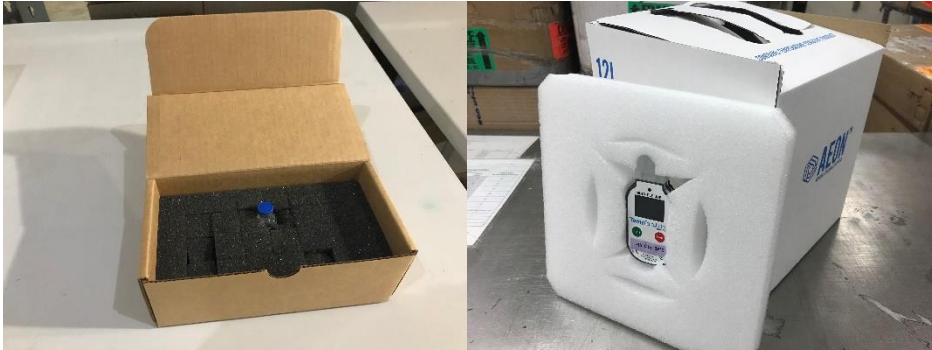
Examples of approved barrier boxes, wrapping/cushioning for vials of vaccine, and temperature monitoring device to be packed directly with vials of vaccine. The packed barrier box containing the temperature monitoring device and vials of vaccine would then be placed in the larger transport box with the cooling agent.
